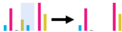
Figure 2. A visualization of interactive deletion, explored in [1]. The sharer selects a region (denoted in light blue) and the activity is replaced with zero values, which is very common in step data.
