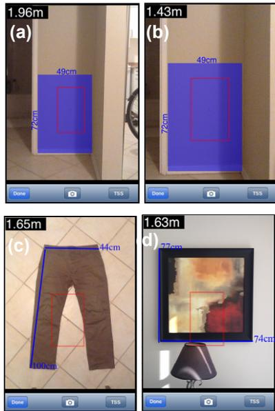
**Figure 5.** Visualized dimension measurement in blue rectangle form at (a) 1.96 and (b) 1.43 m reference depth. The size of the dimension guide area is 49 x 72 cm<sup>2</sup> for both cases. (c), (d) In blue line form. Bottom right TSS button turns on the target signal selector and top left text shows distance to the reference area shown by the red bordered box.
