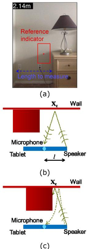
**Figure 4.** (a) The reference indicator shown as a box with red border shows where the distance detection is made. (b) Schematic (top view) for the object far away from the target audio pulse path (solid green line). Distance detection is successful. (c) The object is in the target pulse path and blocks the pulse propagation. The audio pulse different from the target pulse reaches the microphone due to the diffraction effect (dashed line). As a result, unintended distance detection is done.
