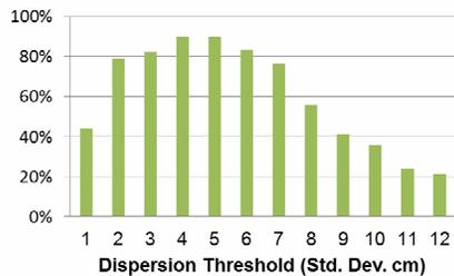
**Figure 3.** Success rate vs. dispersion threshold (in converted flight distance). Success rate is the rate at which the correct pulse signal is selected within one round of forward-backward user motion. At each threshold 109 trial were conducted. The dispersion verification period was set to every 10 flight time detections with a detection rate of 20 Hz.
