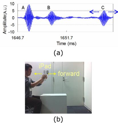
**Figure 2.** (a) Temporal acoustic signal; (A) emitted pulse, (B) downward, and (C) forward direction returned pulse. Pulse C is the target signal pulse reflected by the forward object. (b) User motion in target signal selection. The tablet device is moved forward and backward.
