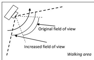
Figure 5: Setup with Rotating Kinects for Increased Field View
