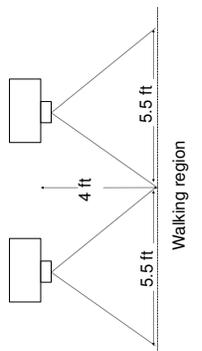
Figure 4: Setup with Multiple Kinects for Increased Field View
