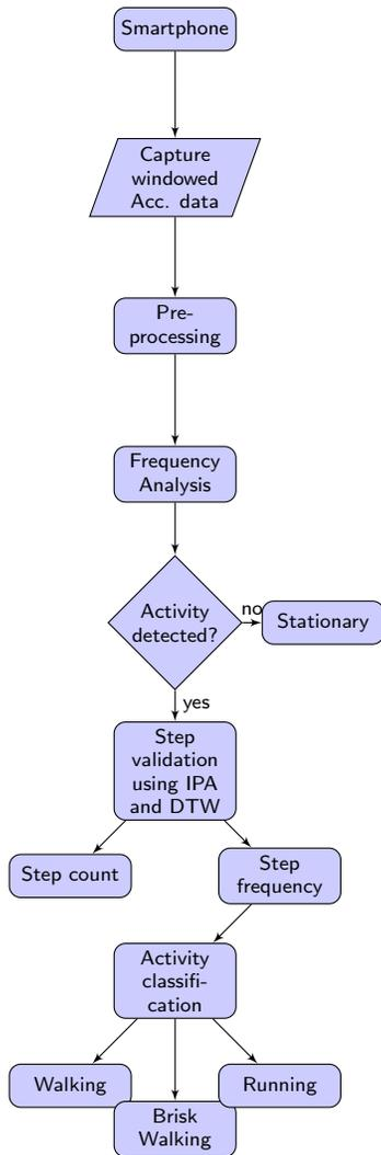
Figure 2: Block Diagram of Activity Classification and Step Count
