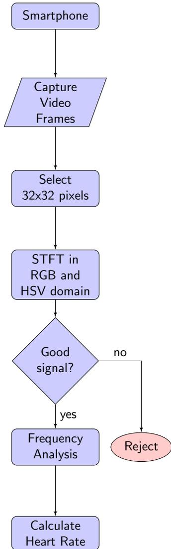
Figure 6: PPG based Heart Rate Detection
