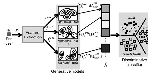
Figure 1: Architecture of our activity recognition method.
