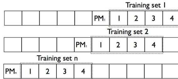
**Figure 1:** Using a sliding window to update the prediction model.
