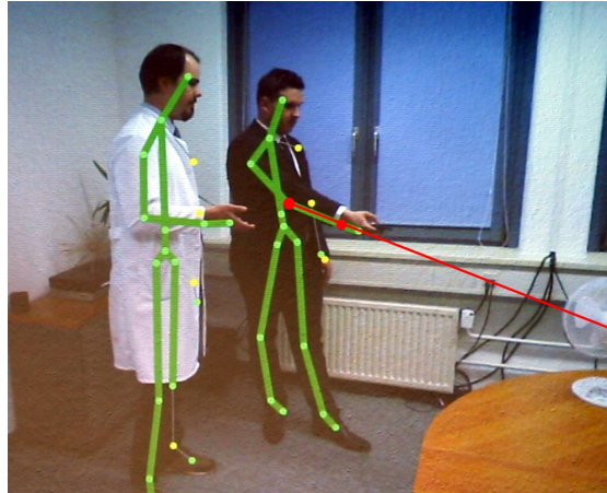
Figure 4: The server uses a Kinect to continuously track the users' skeletons and calculate their aiming direction.
