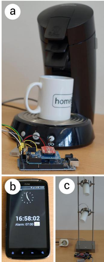
**Figure 4:** homeBLOX smart devices: (a) smart coffee maker, (b) UPnP alarm clock, and (c) smart lamp.
