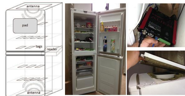
**Figure 1:** System design and deployment of iFridge
