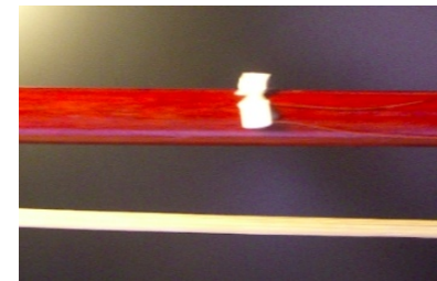
Figure 1: Every 8 cm a ring of SMD LEDs is fixed on the bow. Thin copper wires are used for electrical connection to the battery on the frog.
