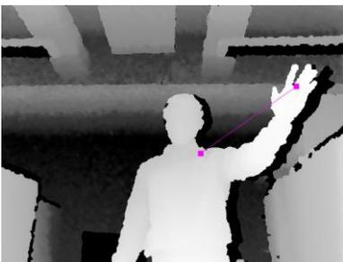
**Figure 4.** Depth image generated by Kinect, also showing the relative distance between the first tracked point and active tracking point.
