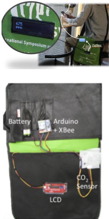
Fig. 1. Measuring CO<sub>2</sub> concentration to estimate the level of crowding.
