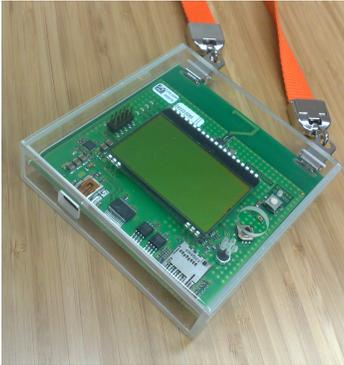
**Figure 3:** The sensor badge we used should become the size of a credit card in the future.
