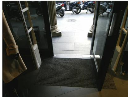
**Figure 2:** Antennas hidden inside the entrance floor mat for EAS.
