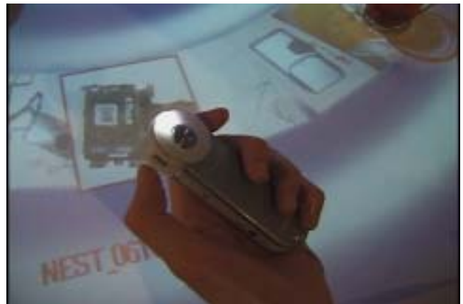
Figure 1. TACT is used for browsing images on a digital enabled table. The white light is slowly blinking during a connection is established.
