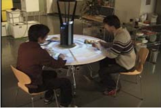
Figure 2. People can share document stored in a file server by operating their TACT devices. Just an intuitive “pointing” operating is enough to establish a wireless connection.
