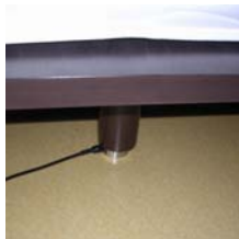
Fig. 1 Conductive textile electrode for measuring ECG in bed
