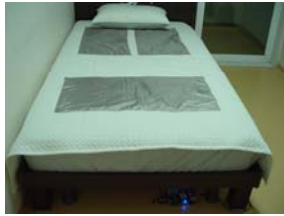
Fig. 1 Conductive textile electrode for measuring ECG in bed
