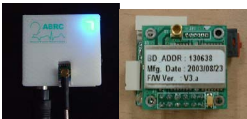
Fig. 3 Magnetic switch and data processing module
